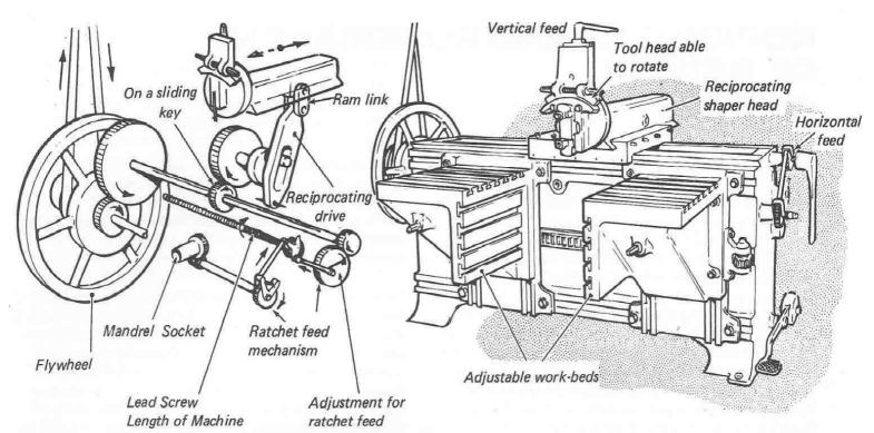
from the front of then machine between the two tables, is the rotating socket which can accept a shaft, called a mandrel, on which work can be mounted. The machine can thereby cause the tool to reciprocate above the mandrel, but parallel to its axis, whilst the mandrel is slowly rotated. It was thus possible to shape a cylindrical form, a facility which was used to produce splined bushes. (Splines are a form of teeth, placed around a shaft, which are parallel to its axis).
