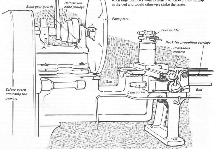
The drawing shows a horizontal bar in the foreground similar to a handrail in appearance. This, in fact, is a belt-striker control, extending just over halfway along the machine, and it eliminates the need for the return of the operator to the headstock each time a start or stop is required. Owing to the machine's length, this control is more than a convenience; it is an essential item.
