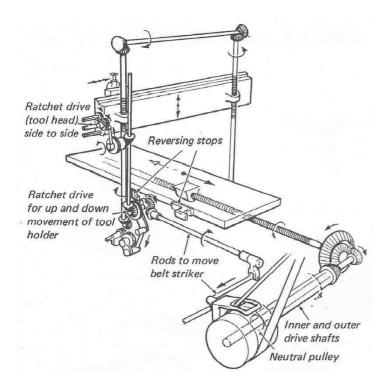
The lead screw is arranged always to take only tension loads. Bearings to accommodate axial thrust exist at each end of the screw. The one at the drive end carries loads due to cutting, and is of the multi-collar type, lubricated manually. The machine can accommodate a stroke variation of 18in up to 11ft 6in approximately.
